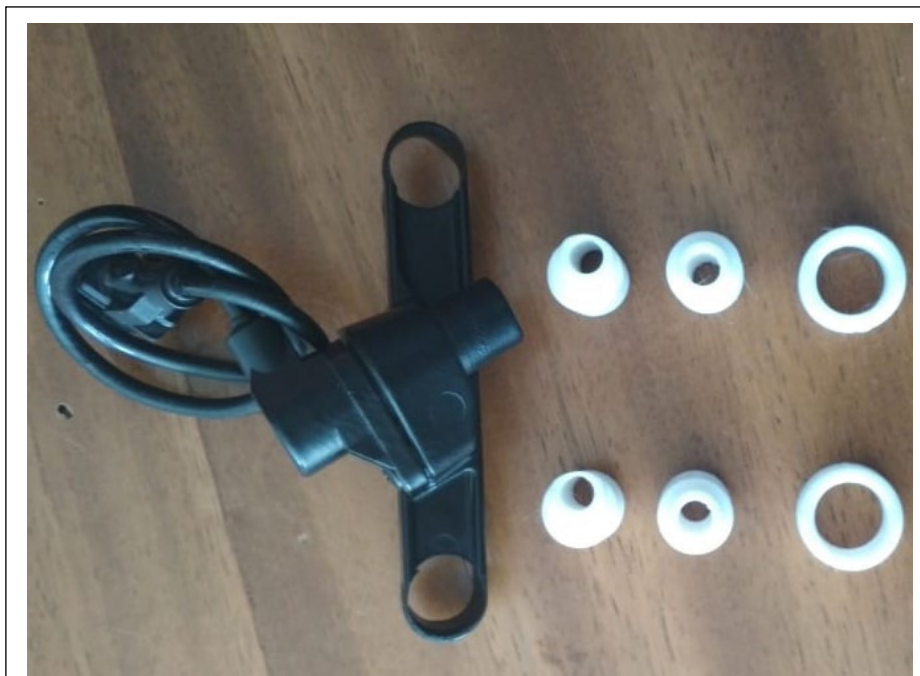
Figure 2 - Components used to change the fuel injection point (1. crankshaft position sensor, 2. eccentric bushings to modify the sensor attachment position, 3. centered bushings to simulate the original condition of the phonic wheel reading by the sensor, 4. common bushings for fixing the other bushings on the tractor engine).
