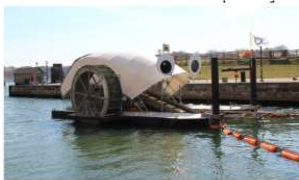
Imagem 2 - Mr. Trash Wheel. FONTE: Waterfront Partnership / Mr. Trash Wheel. Trash interception – Mr. Trash Wheel in operation.
